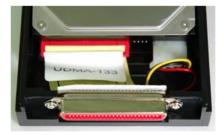
Place and lock the HDD tray to DVR-400. Power on the DVR-400, the DVR-400 will now automatically detect and format the new disk(s).
